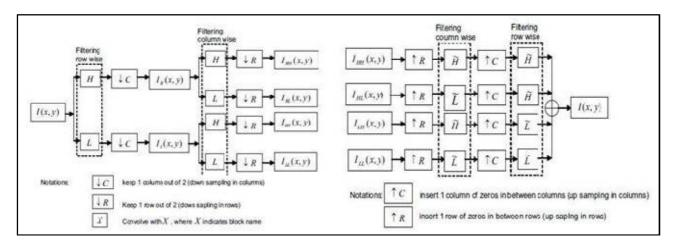
Figure 1: One Level Of 2-D Image Decomposition[7]
