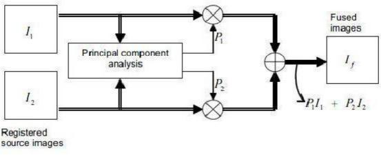
Figure 4 : Information Flow Diagram Of PCA
